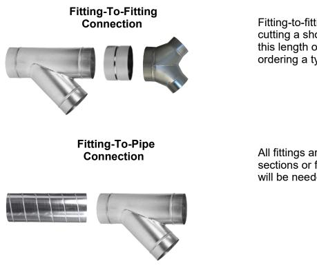
Fitting-to-fitting connections can be made by cutting a short length of spiral pipe and using this length of duct as a female coupling or by ordering a type COU2 female coupling.
