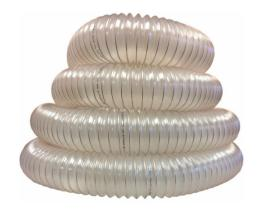
U20-AS antistatic, light weight, highly flexible, compressible (3:1), abrasion resistant, microbe resistant and flame retardant flexible hose. Lighter weight, lighter duty version of the U30-AS. Flame-retardant according to DIN 4102-B1. Permanently antistatic wall: electrical and surface resistance <109  $\Omega$
