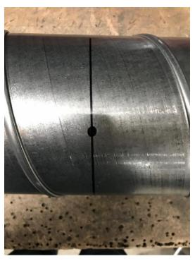
We are regularly asked how easy is it to cut spiral pipe. Quite simple, scribe line, drill and cut. See <a href="attached PDF">attached PDF</a> for more information.
