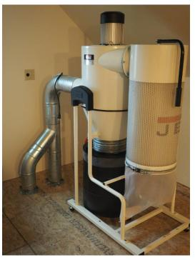
2 hp Jet cyclone dust collector located in the attic. I plan to come down through the attic floor into the work shop and then span out to 2 or 3 inlets. I will be traveling from Ohio to Massachusetts by way of Connecticut and want to pick up this material." Two weeks later he arrived to pick up his ductwork. With the holiday's just weeks away, he will be stopping again on his way to visit his family and picking up some flexible hose to finish up his final connections.
