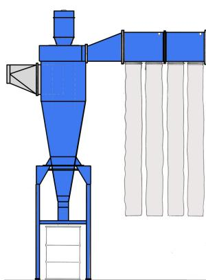
Since most woodworking dust contains coarse-sized and fine-sized particles, a two-stage dust collection system is generally recommended. A two-stage dust collector consists of a first stage cyclone, a blower and a second stage after filter.
