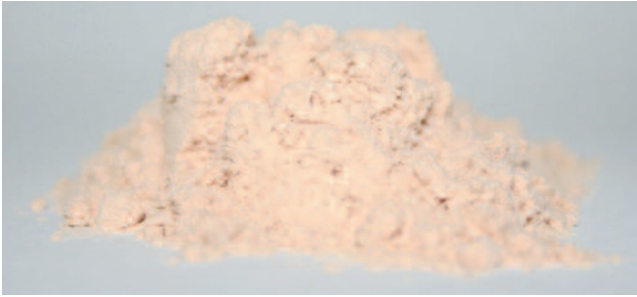
This wood flour is the “fuel” for the fire, as shown in the dust explosion pentagon.
