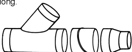
Fitting-to-Fitting connection with short piece of spiral pipe.
