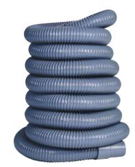
**Constructed of:** Longitudinal and helical polyester fibers bonded to a final layer of PVC reinforced with a spring steel wire helix. **Color:** Grey. **Standard Length:** 25 ft. **Temp. Range:** -20<sup>o</sup>F to 150<sup>o</sup>F.
